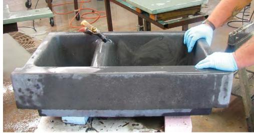
When you place a piece of foam on day-old concrete you end up with a dark spot under the foam. The trapped escaping moisture darkened the concrete. This is why you should not seal your concrete the day after casting. The escaping moisture may compromise the sealer. Time is not the best judgment of when you can seal, moisture transmission is.
