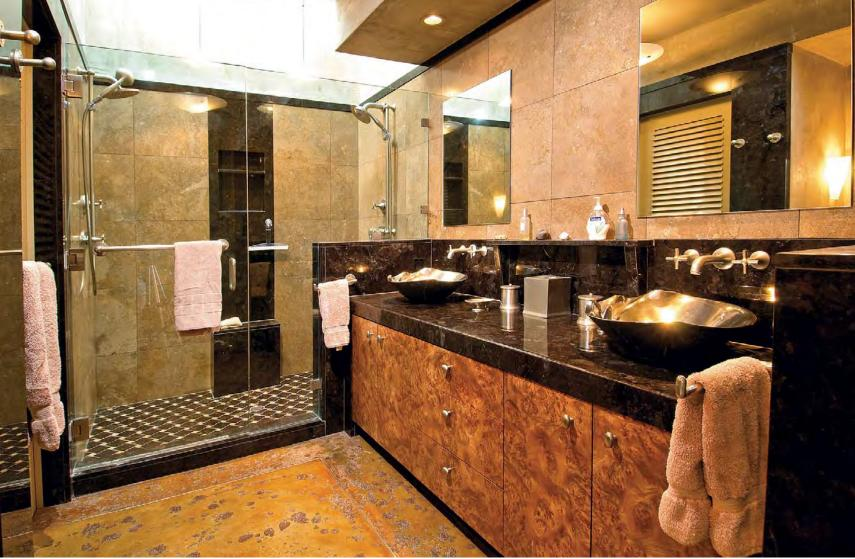
The visible craters in the bathroom floor were created by using a turkey baster full of retardant to create a random-looking pattern.
