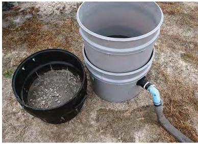
Using three stackable chambers to filter wash water, The Sludge Buster provides particle separation as well as chemical treatment.
