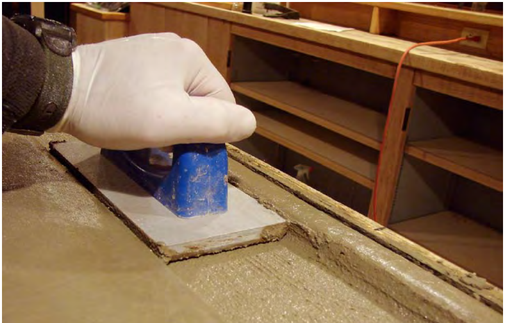
I made a tool with the same profile as the drink rail to finish it.
