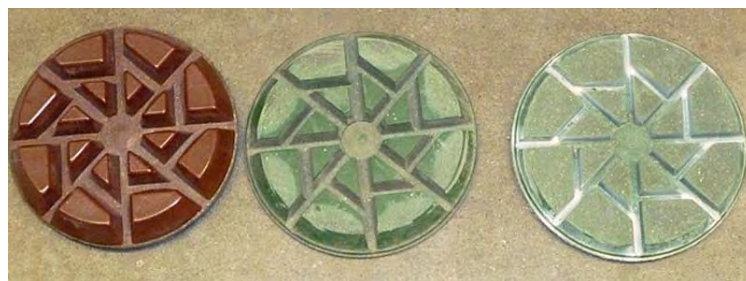
Resin bond diamonds. Left to right: sealed and unopened; partially open with center untouched; open with visual sparkles. The green diamond on the right is open and ready to cut, and the red diamond on the left is not.
