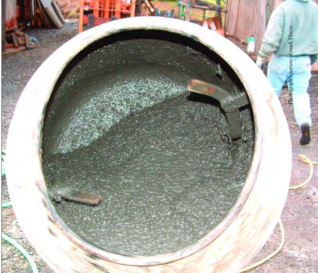
The black in this mix is Davis Colors Black 860, an iron oxide pigment.
