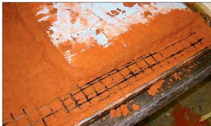
C-Grid is used around a sink hole.
