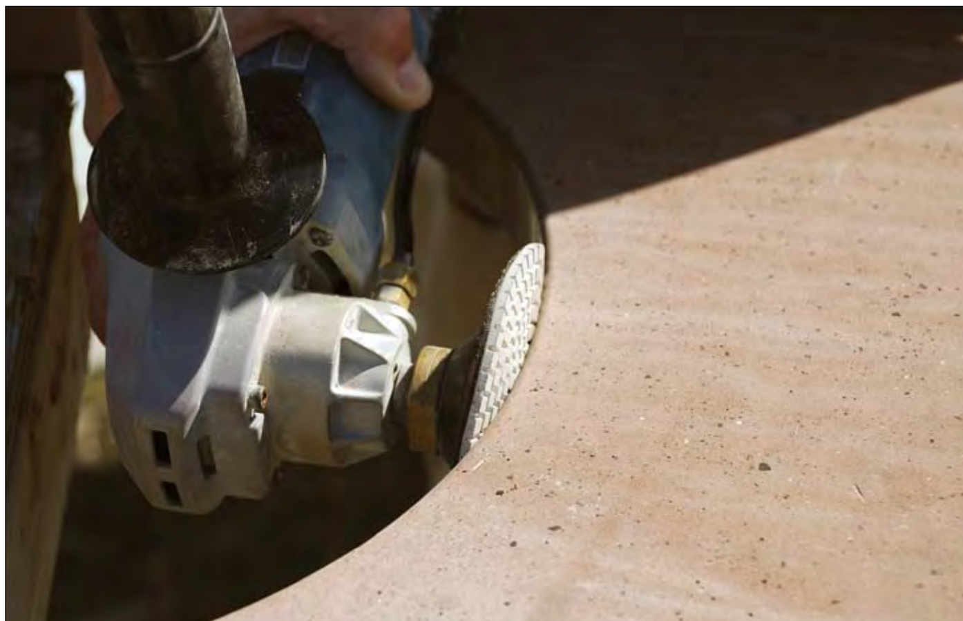
This Makita PW5001C wet polisher/grinder is being used with an alpha 3-inch flexible backer pad and a 4-inch polishing pad to polish the inside of an under-mount sink. The undersized backer pad allows the outside of the pad to bend and get into hard-to-reach places.
