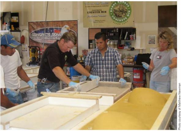
Matthew Newman shows how to fabricate concrete sinks in a precast form during a Vision Concrete Institute workshop.
