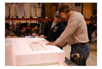
visible imperfections, which, if not treated, would end up transferring to the concrete finish. A protective coating is then peeled away from the base to expose the smooth, glass-like working surface.
