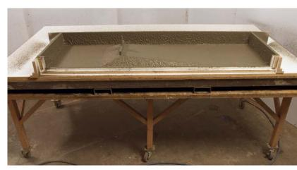
The mold, completely sprayed with the face-coat mix.
