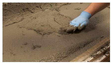
Step 8: Wait for the face coat to become stiff, but not dry, and then apply a thin application of the vertical back coat, an application also known as a scratch coat. Add a small amount of water, if needed, to thin the consistency of the back coat and make it more workable. Applying this thin scratch coat helps to prevent any air pockets from forming between the face coat and the back coat.
