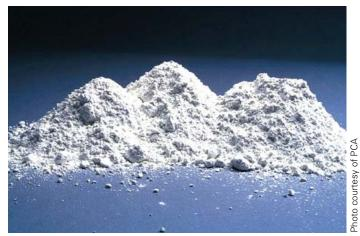
There are only slight chemical differences between gray and white portland cement. Manufacturers usually control the color of white cement by limiting the amount of iron and manganese oxides.
