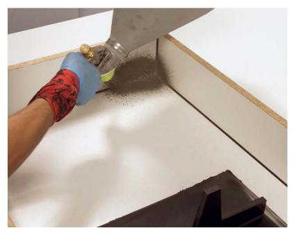
Step 5: Spray. Begin by spraying into the corner of what will be the front edge of your piece. Your spraying technique will be the primary factor in the quality of the finish. When spraying GFRC, you always want to spray into a corner and work your way back, spraying into the face coat you've already sprayed. By doing this, you compact the face  $% \left( 1\right) =\left( 1\right) \left( 1\right) \left$ coat and force out any air bubbles. This is the secret to a superior finish for GFRC.
