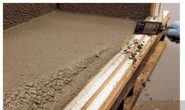
Step 11: Scrape the excess face coat off any walls where the self-consolidating back coat will be poured up to them. This will ensure consistent, accurate thickness in your piece.
