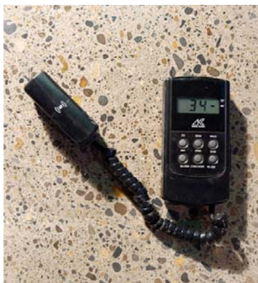
Three gloss readings from the same exposed-aggregate concrete sample. Note the range.
