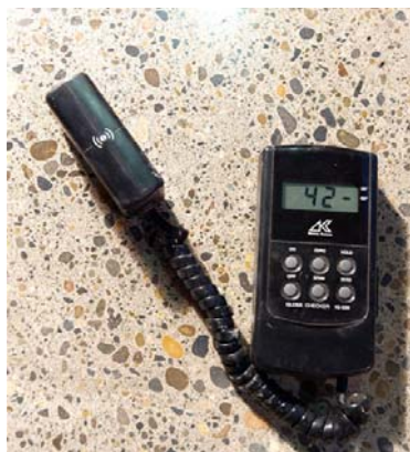
Three gloss readings from the same exposed-aggregate concrete sample. Note the range.
