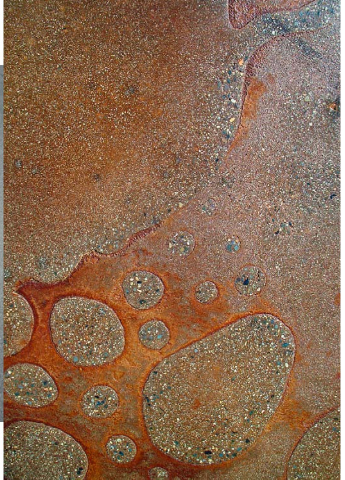
When raw embossed concrete is light diamond-sanded with soft pads, stained and sealed, it becomes quite refined.
