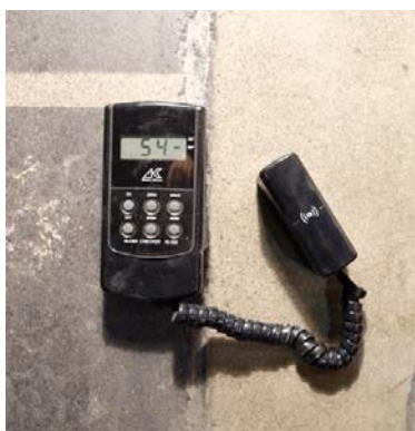
Three gloss readings from concrete with a salt-and-pepper look.
