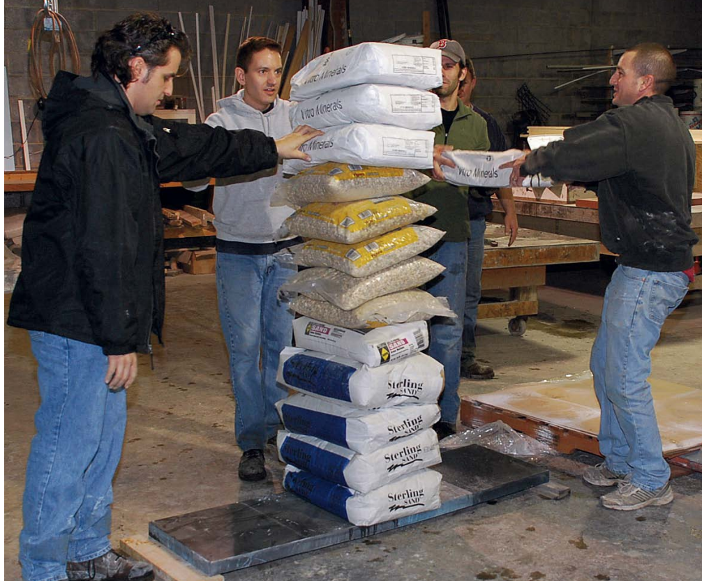
A scrim-augmented GFRC beam bearing a load of 835 pounds.
