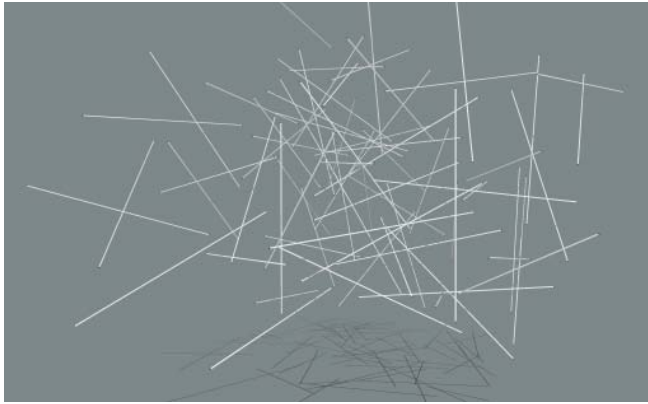
Random three-dimensional reinforcing occurs when fibers are mixed into the concrete, which is then simply poured into forms.
