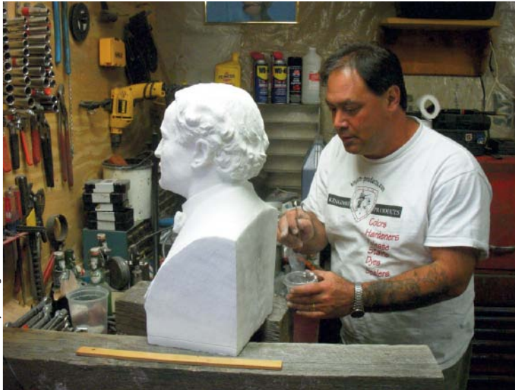
Bart Sacco does minor touch-up work prior to installation. He is using a slurry to restore a clean edge to the piece because it was chipped after demolding.
