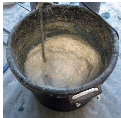
13-mm AR glass fibers being mixed into GFRC backer.
