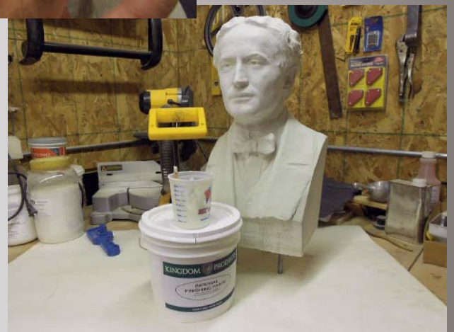
Imperial Finishing Paste, a compound from Kingdom Products, is used to fill any voids or imperfections in the model.
