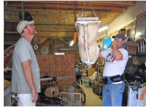
Removing the cured piece from the vacuum box.
