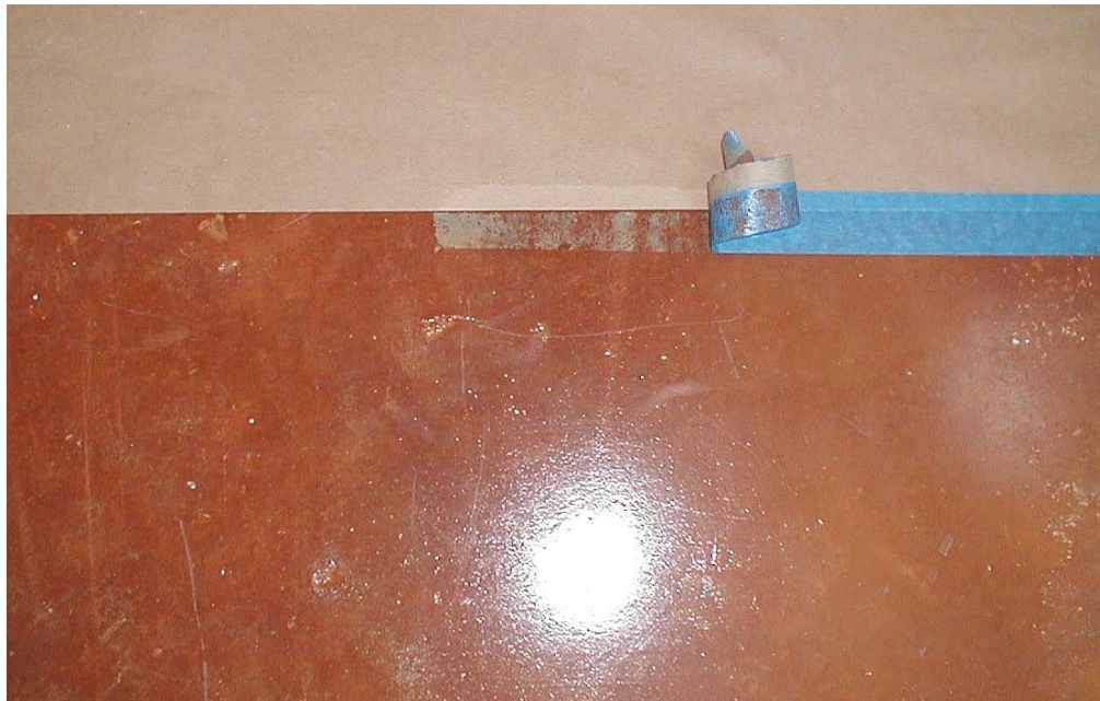
An example of blue painter's tape pulling up and damaging acrylic sealer and acid stain.
