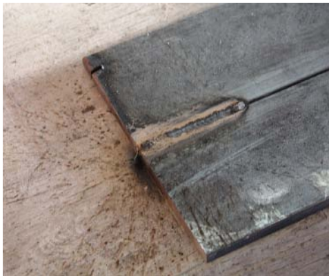
A typical weld from a flux-cored arc welder. This is residue left behind by the gases and flux. It is easily removed with a wire brush and minor scraping.
