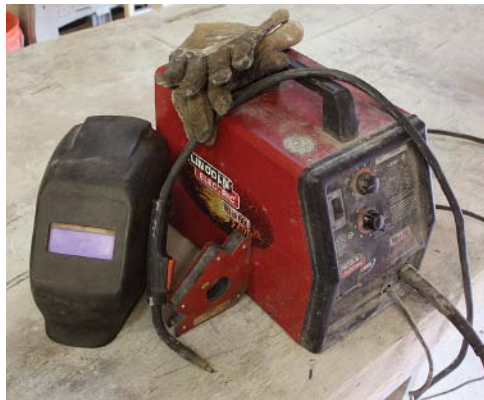
The basics to get started: flux-cored arc welder (with MIG conversion), welding gloves, welding mask (auto-darkening recommended) and magnetic squares.
