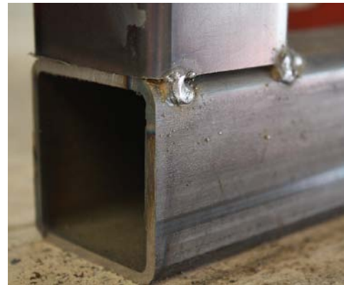
Make sure all four corners are properly tacked after squaring before running a full weld. This will ensure the steel's placement. If not tacked, the material will tend to bend towards the point of the weld, resulting in a very out-of-square bond. Usually, this cannot be fixed without breaking the weld and starting over.
