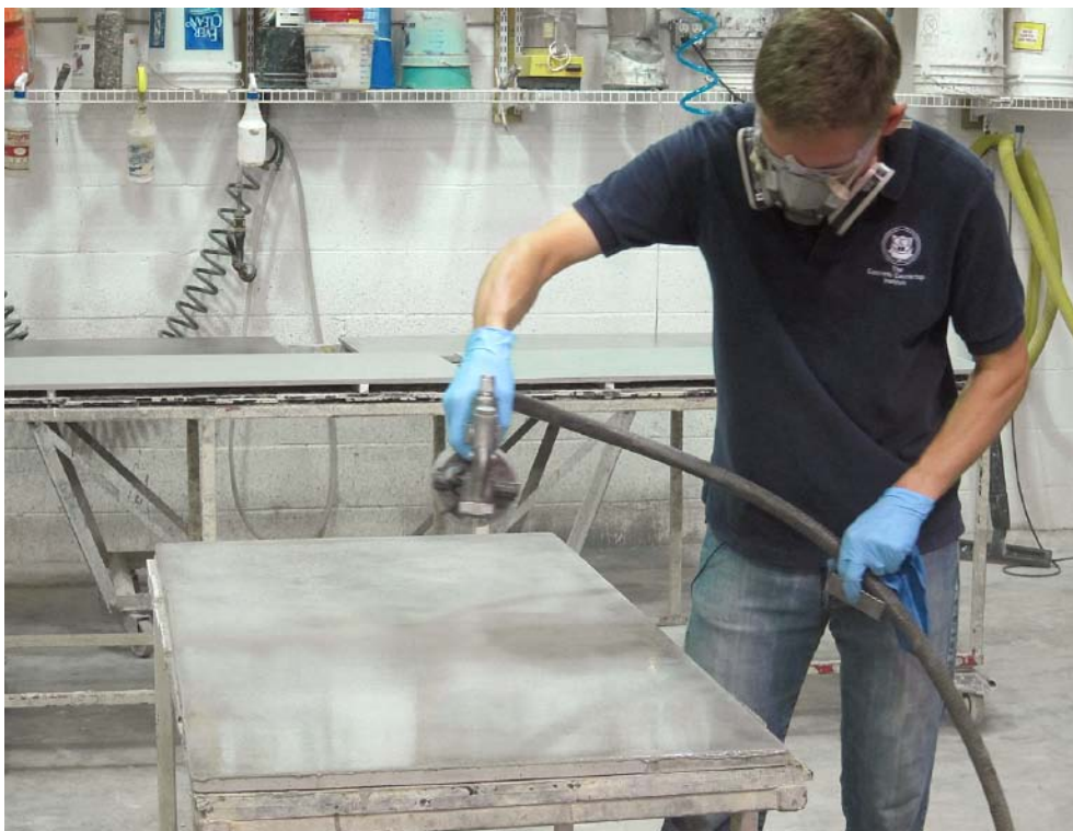
Jeff Girard applies a water-based urethane sealer with an HVLP spray gun.
