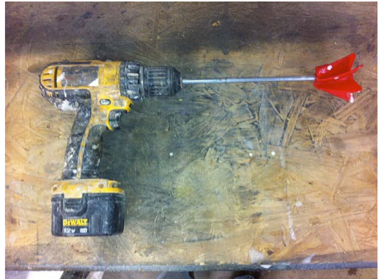
An example of the drill and mixing blade Jeff Kudrick uses to mix sealers.
