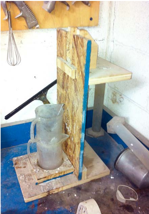
A useful tool tip from the author: This homemade mixer stand will hold down the trigger on a drill, allowing you to take notes on your working conditions while your sealer is mixing.
