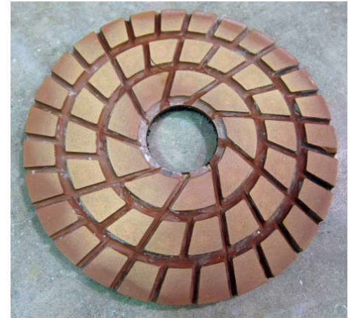
Cupping caused uneven wear on this thick pad.
