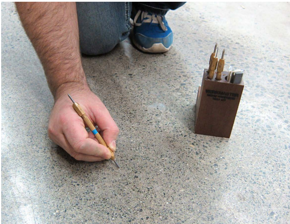
A Mohs hardness test kit from WerkMaster contains four picks. The picks are color-coded to link them with regions on a map of the United States showing the typical hardness of concrete in each area. Also included in the kit are a sharpening tool and three test plates to help contractors master scratching technique.
