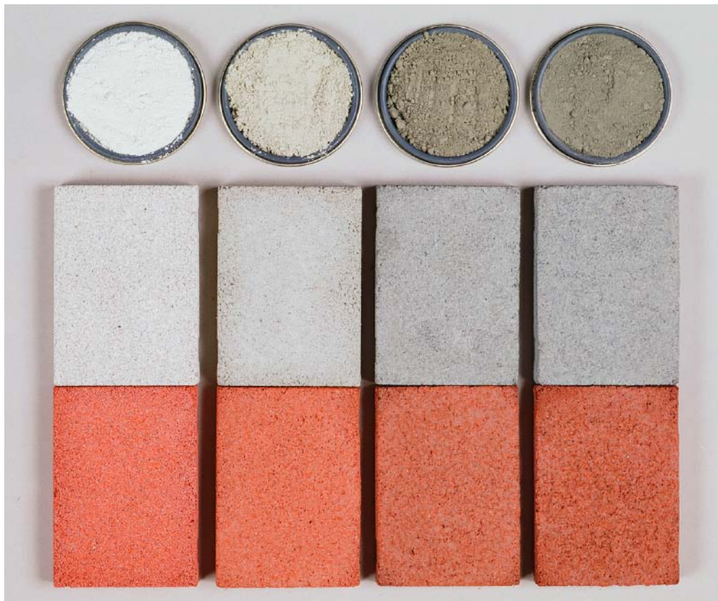
These samples show how cement color can affect concrete's appearance. Cement samples at the top range from white to dark gray. The cements were used to make the uncolored and colored concrete samples below them.
