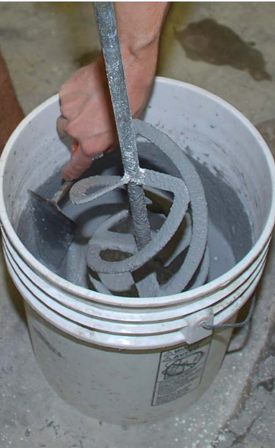
A drill mixer being used to make a small batch of glass fiber-reinforced concrete in a 5-gallon bucket.
