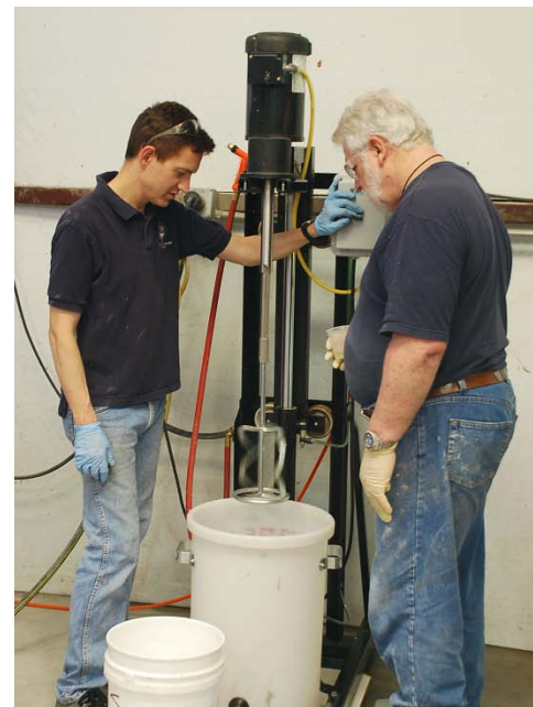
The GFRC Mini Mixer from RimCraft Technologies Inc. is a small, high-shear mixer with two speeds and a claimed 150-pound batch capacity.
