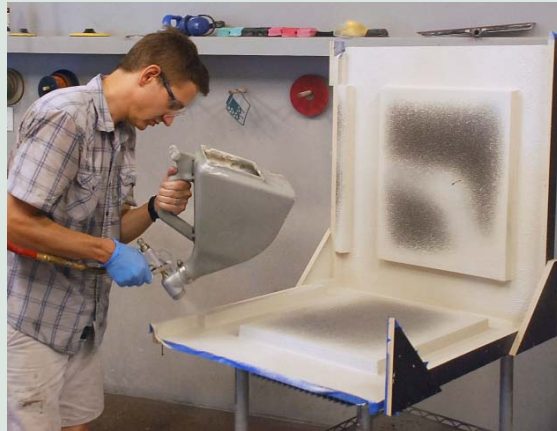
Spraying the mist coat into each form half.
