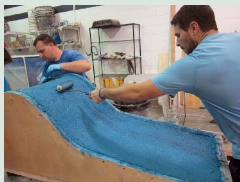
Rolling and compacting the backer in thin layers.
