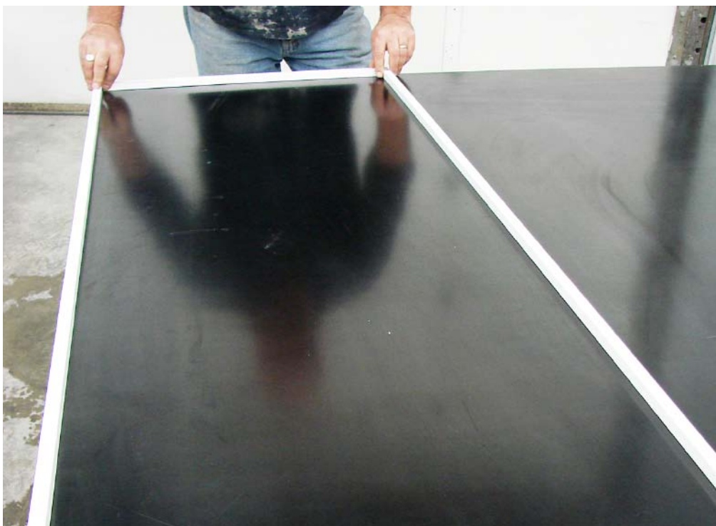
Steel casting tables with two-sided tape and plastic rails make for quick, clean, efficient project setups.
