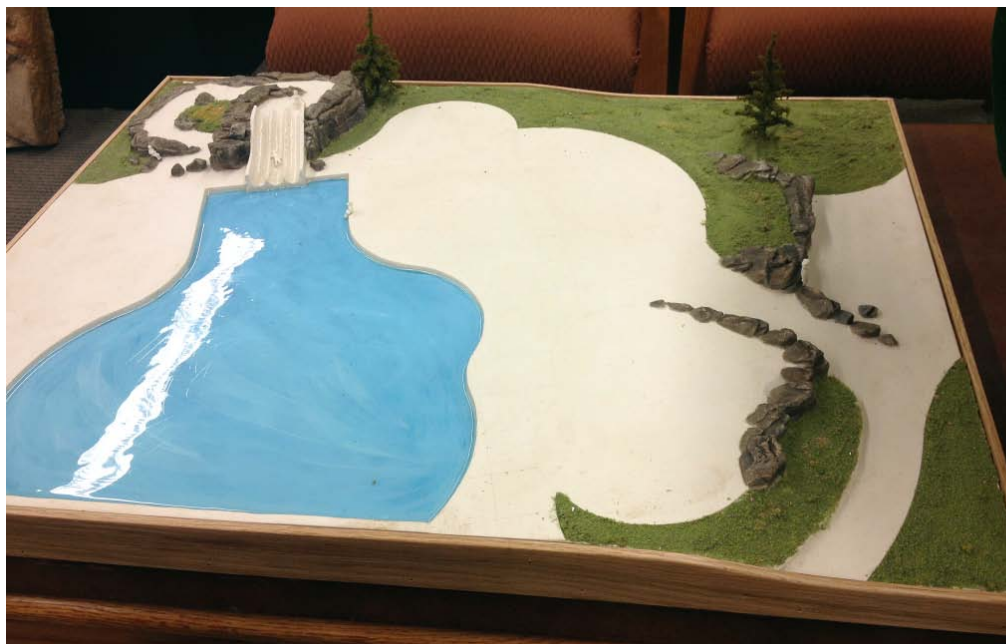
A maquette prepared by Colorado Hardscapes Inc. to propose the layout, size and form of rockwork that their division, di Giacomo Inc., would build at an upgraded outdoor aquatic center in Broomfield, Colorado.
