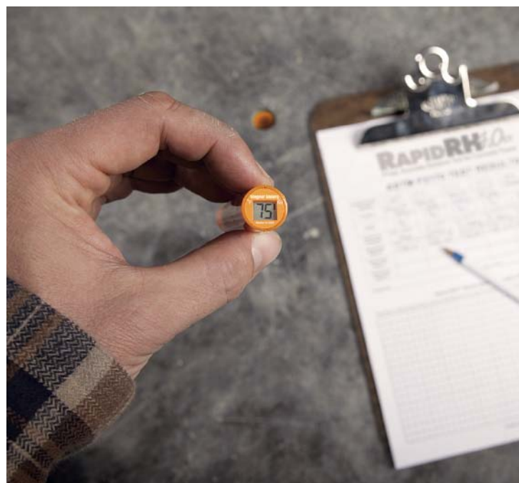
A Rapid RH meter measures the moisture content of concrete.
