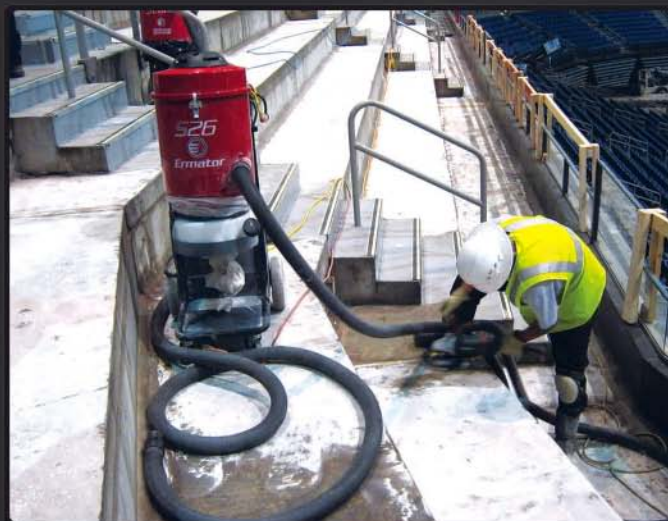
Twin motor single phase (120V or 230V) dust extractor
