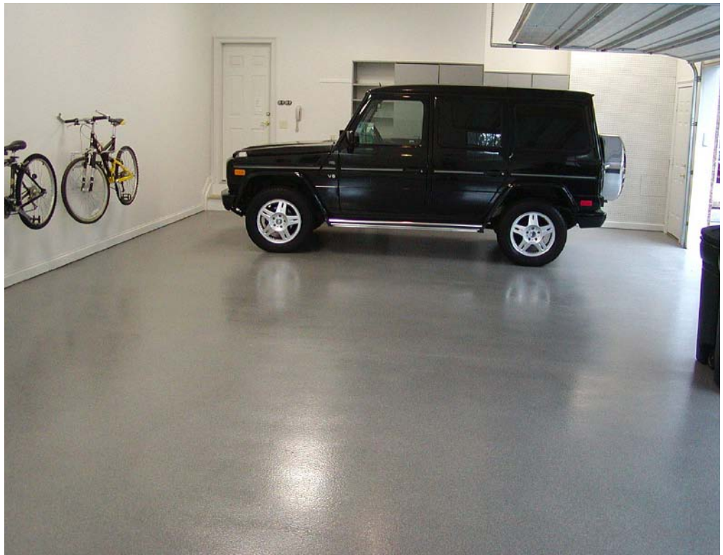
Key Resin president Jeff Cain says that broadcast quartz makes more sense in garage settings, where a troweled system would be more costly and require more skill to install.
