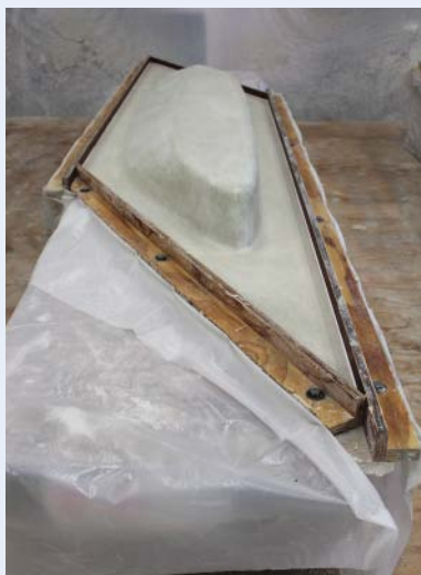
The GFRC cladding elements of the Broad Museum were produced using polystyrene foam forms. A coating was applied to the roughed-out forms to provide a smooth, hard surface.
