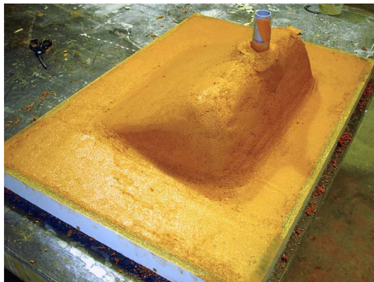
Here's a mold for a hand-packed ramp sink.
