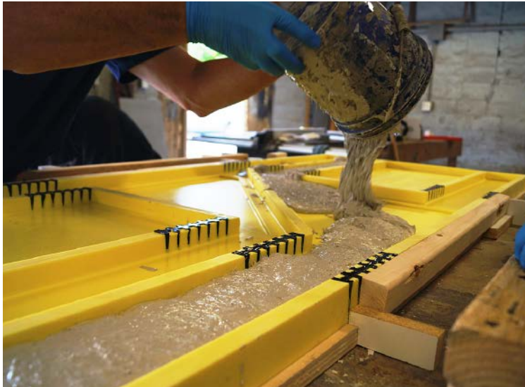
Sheets fills in the rubber mold for an end table with self-consolidating GFRC mix.
