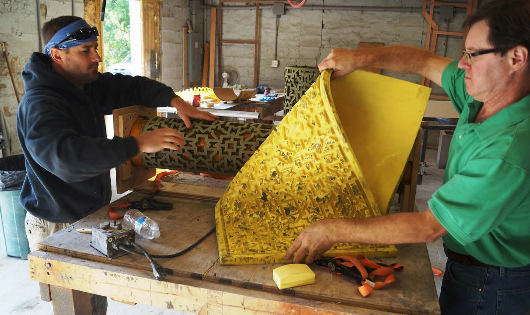
Eric Schaeffer of Majestic Concrete Design and Bill Sheetz of Polytek Development Corp. strip a lattice panel from a cylindrical form. Photos by Dennie Boyer, Polytek Development Corp.
