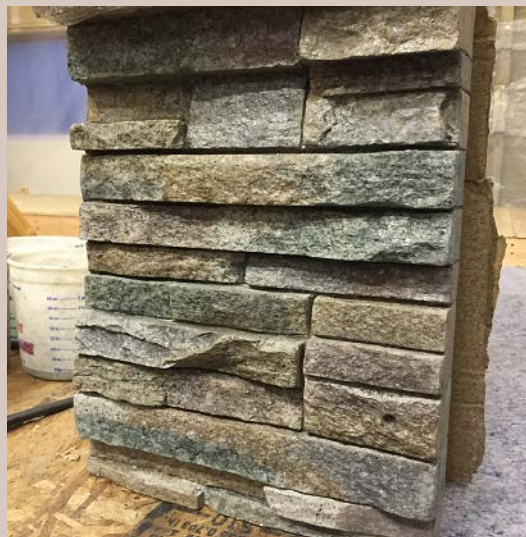
CMJ can cast lightweight sheets of veneer stone in a host of sizes and finishes, including fieldstone (left) and stack stone.
