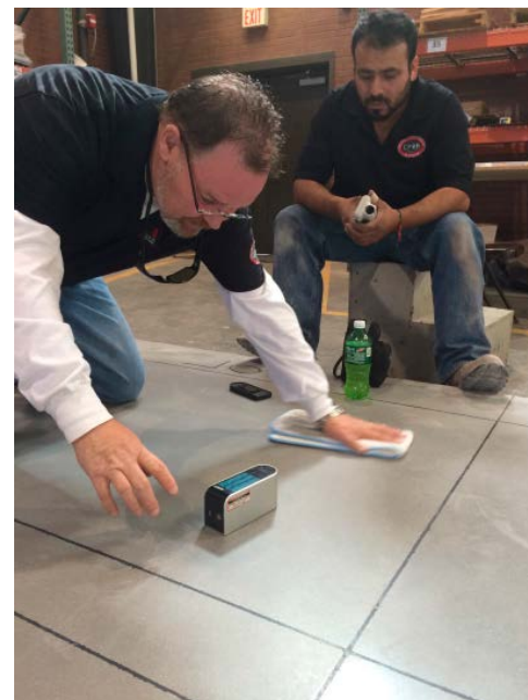
The CPAA measured the gloss of all 48 individual squares to ensure the gloss levels as defined by the CPAA were met.
