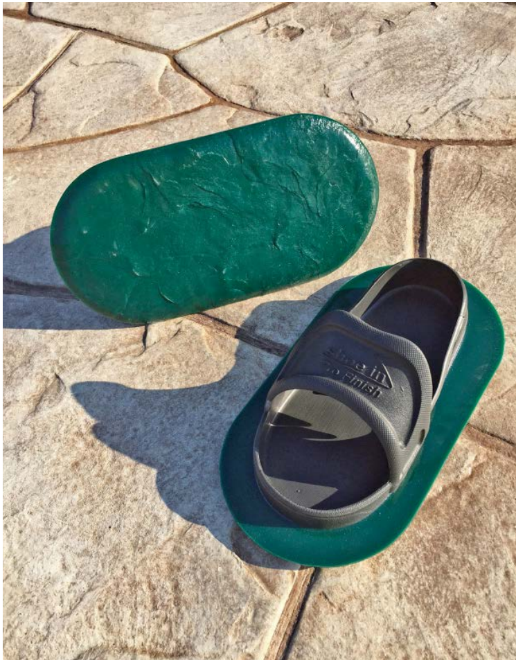
Texture shoes allow a crew to get out on a slab as soon as possible to begin stamping. The stamping in this photo was done without a tamper.
