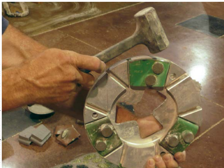
There are many different types of diamond tools, including backing plates that play a supportive role in the polishing process.
