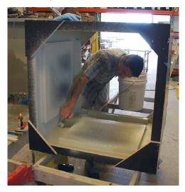
Because the Caymans are very hot, I chose to spray first and then assemble the two halves instead of spraying first and then assembling four individual sides. The work must be done very fast, and preassembly makes it much easier.
