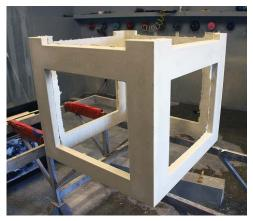
The inside of the table wasn't finished to the same degree as the outside. While the outside didn't have exposed fibers, the inside did. This didn't matter since the inside wasn't going to be very visible. For the inside, I used a pneumatic diamond polisher with a 50-grit pad, then 100 and finally 200.
