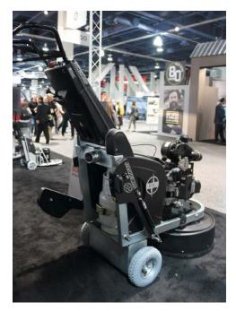
**HTC** (www.htc-floorsystems.com) launched its first propane grinder at the show, the 800 RXP. Except for its power source, it's almost identical to the popular remotecontrolled 800 RX electric model but goes one better. Designed with ergonomics in mind, the new four-head 800 RXP offers up to 50 percent higher productivity. A floating grinding cover helps reduce airborne dust. Expect more propane products to follow, a spokesman says.
