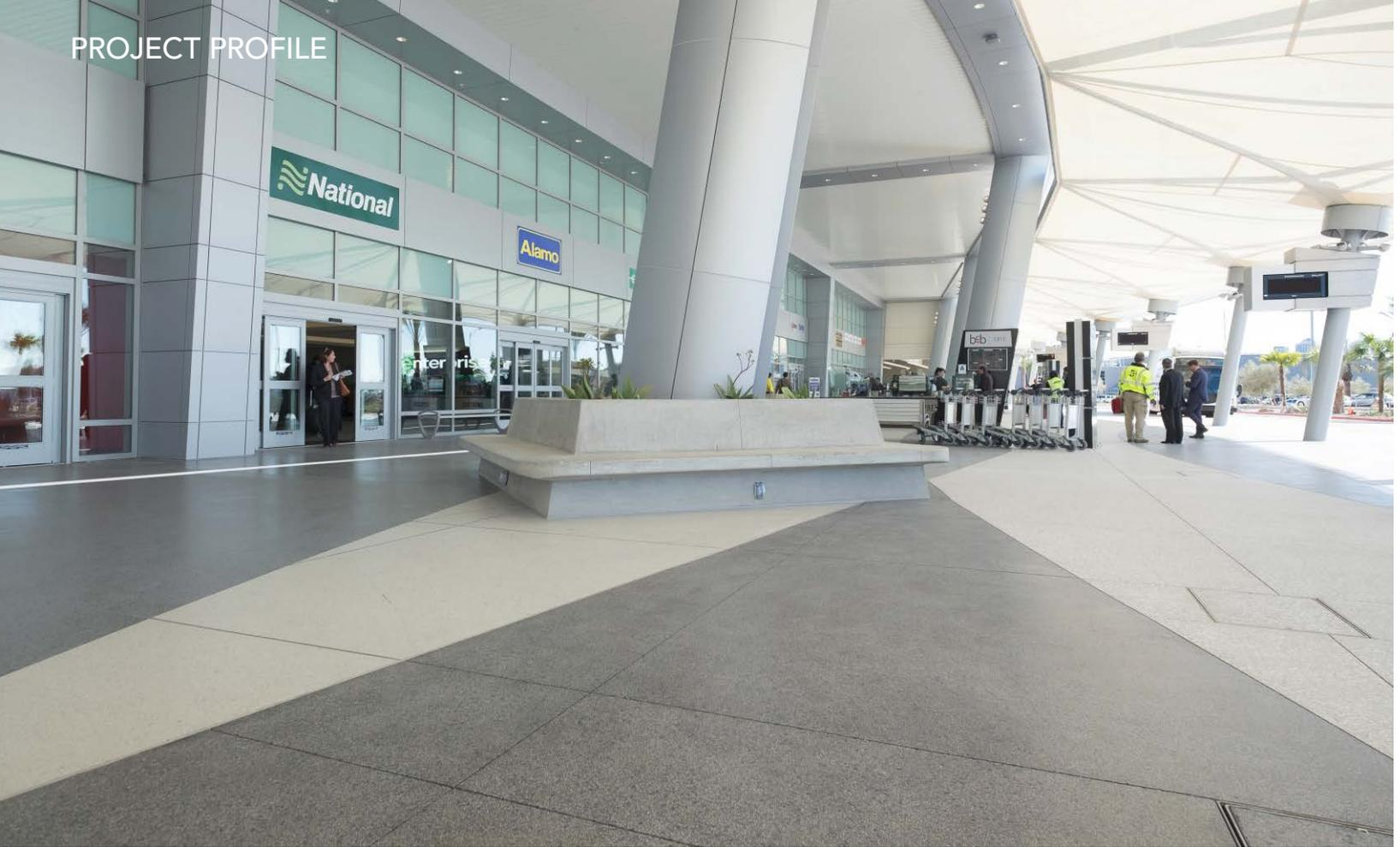
The area directly under cover by the building is terrazzo and the areas outside that to the bus canopy are architectural concrete. So the dark and light sections to the left are terrazzo while the dark and light sections to the right are honed concrete. T.B. Penick also made the poured-in-place concrete bench planters.
