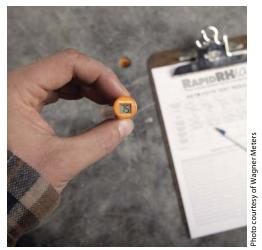
A popular invasive testing device, Wagner Meters' RapidRH will deliver fast and accurate moisture readings that easily comply with ASTM F2170.
