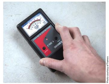
Tramex CME4 can be used to conduct a nondestructive moisture content test as per ASTM F2659.
