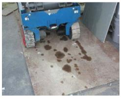
I also ask my GCs to specify one area where lifts must be parked to charge each night. They can cover this area and then check all the lifts each morning before work starts. I've seen diapers get so full of oil that they fail and dump puddles of hydraulic oil onto the floor. Inevitably you'll have oil spots on the floor, especially if you have a larger project with a long duration.
