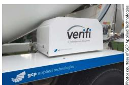
Technology is even reaching ready-mix trucks. With Verifi, there's no question that batch of concrete won't be at the correct slump when it reaches the job site, or be the same as the load before and the load after.
