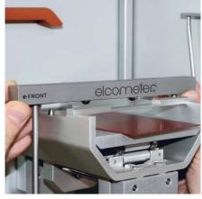
accurate, repeatable results. Simply fit the pendulum onto the loading pins, load the sample and close the door. The pendulum automatically moves to the start position, the sample table rises and the test begins.
