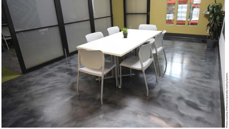
Westcoat's lunchroom at the company's headquarters has a plywood substrate that was transformed into an epoxy floor with the ALX Interior system and Liquid Dazzle.
