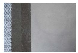
This sample shows a plywood substrate transformed to a concrete surface with Westcoat's ALX Interior system.
