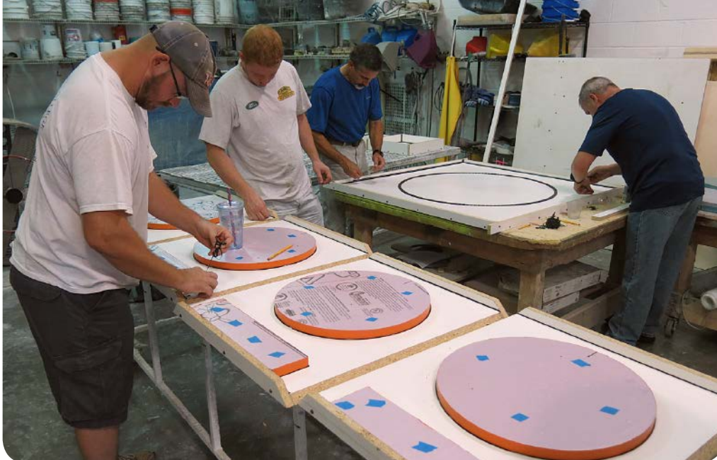
For production casting, plastic is just one of several materials that offer consistency, quick cleaning and assembly.
