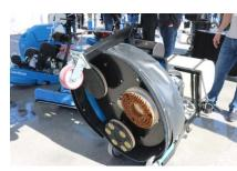
Also in Aztec's procession was the versatile Refresher (above), a propane-powered machine that can be used to strip, deep scrub, hone, polish and burnish concrete and terrazzo floors.
