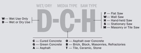
To help contractors determine which saw blade is right for a job, the Concrete Sawing and Drilling Association has devised a classification system that applies to diamond saw blades 12 inches in diameter or larger. The code, which consists of letters placed in three positions divided by dashes (i.e., X-X-X) will be permanently imprinted on each blade.
